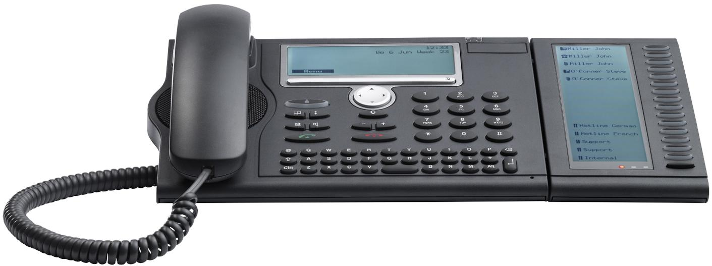
Up to three display extension modules can be connected to the 5380 Operator. The additional keys can be individually programmed and depending on requirements can be allocated either functions or numbers of important contacts.
